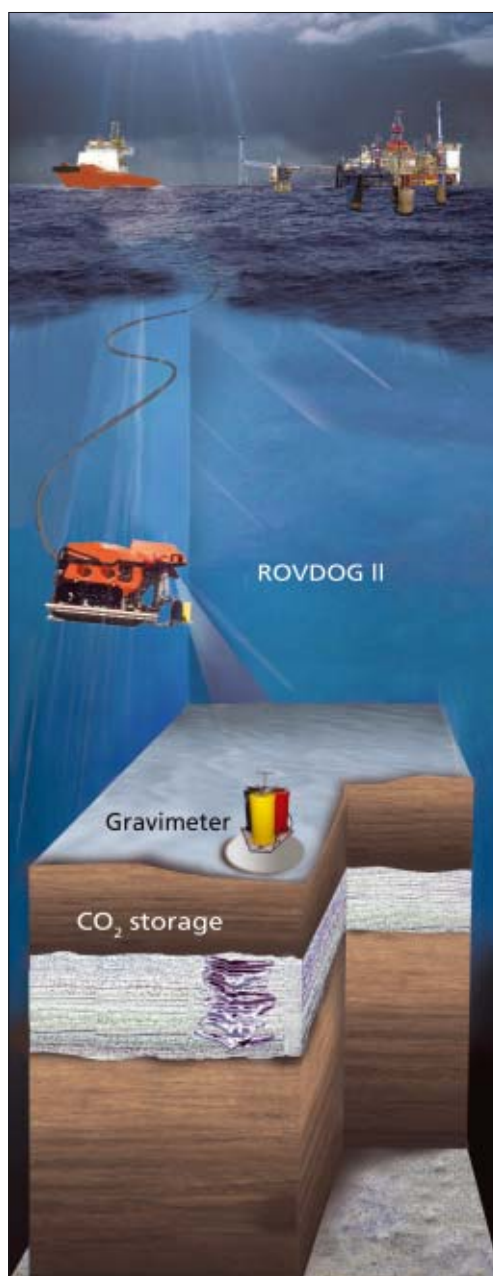
Principle of seafloor gravity surveying. The Remotely Operated Vehicle - ROVDOG II - lowers the gravimeter onto concrete blocks placed on the seafloor (Illustration: Erik Hårberg and Johnny Schumann.)
