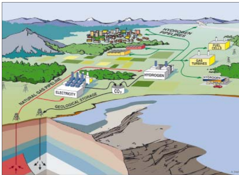
Cartoon illustrating how natural gas can be used to manufacture two CO 2 -free energy carriers - electricity and hydrogen. Note the CO 2 capture plant from which the CO 2 can be injected into subsurface formations for long-term storage and/or CO 2 -based improved oil recovery. (Illustration: Arnfinn Olsen and Olav Kårstad, c 1980.)
